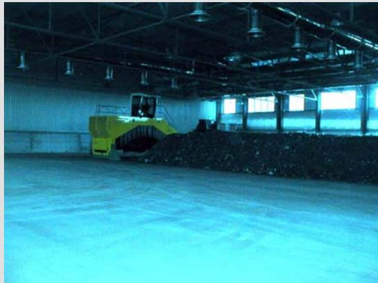
This is then followed by a 45 day curing stage which takes place in a covered (i.e. with a roof) but not fully enclosed area. Overall, the retention time in areas provided with odour treatment systems is 3 weeks. The odour treatment system is the patented HerHof technology LARA (self-regenerative thermal purification of air).
